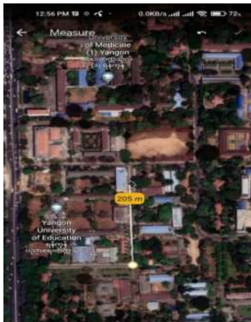
Figure 17 Measurement of range at stable ESP_NOW communication range
